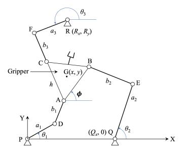
Fig. 4. 3RRR planar parallel robot.
