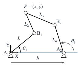
Fig. 2. Five-bar planar parallel robot.
