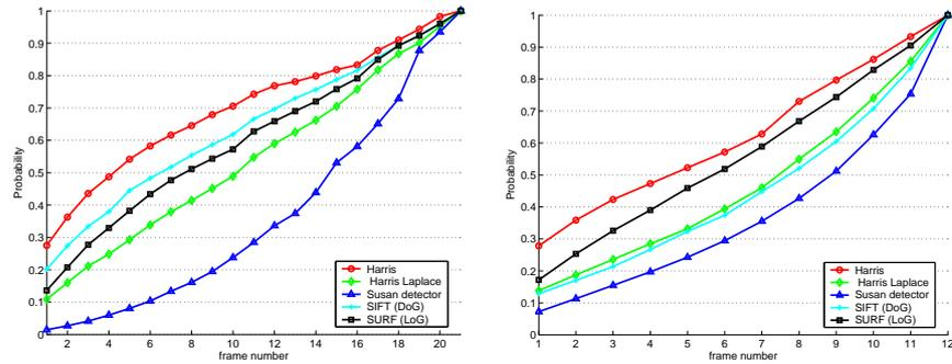
**Fig. 5.** The figures show the probability of a point being detected in the last frame given that it was detected in the frame  $i$  of the sequences: left with changes in viewpoint, and right with changes in scale.
