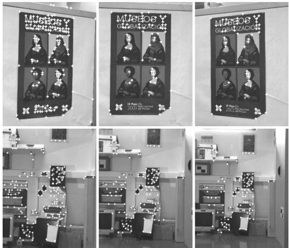
Fig. 4 The top images are examples of a planar object under different changes in viewpoint. The bottom images depict a 3D scene under different scales. These are the first, the central, and the last image of a sequence of 21 images (viewpoint transformation) and of 12 (scale transformation). The tracked points are indicated by white marks
