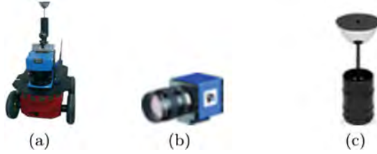
Fig. 1. Real equipment: (a) Pioneer P3-AT mounted with omnidirectional camera, internal odometer and laser range finder; (b) CCD FireWire DMK21BF04; (c) Eizho Wide 70 Mirror.
