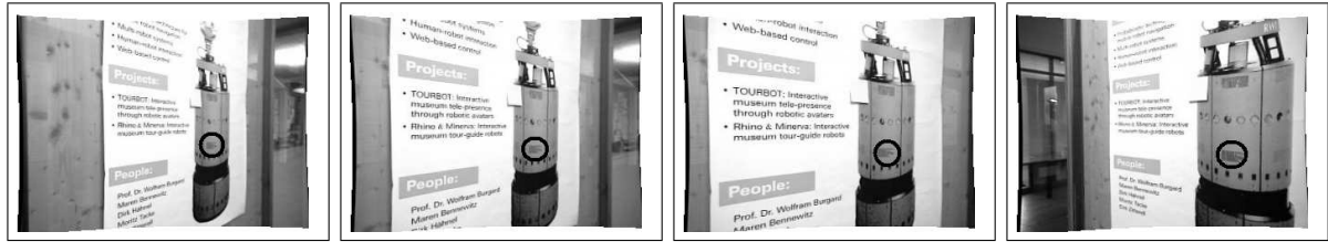
Figure 1: The images depict the same landmark (marked with a circle) viewed from different viewpoints. The squared Euclidean distance between consecutive images is between 0.03 and 0.06. In contrast to that, the squared Euclidean distance between non-consecutive images is between 0.3 and 0.4, which is around one order of magnitude larger.
