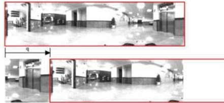
Fig. 1. A robot rotation in the ground plane produces a shift in the columns of the panoramic images captured.
