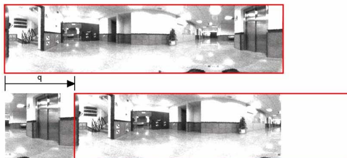
Figure 2. A robot rotation in the ground plane produces a shift in the columns of the panoramic images captured.
