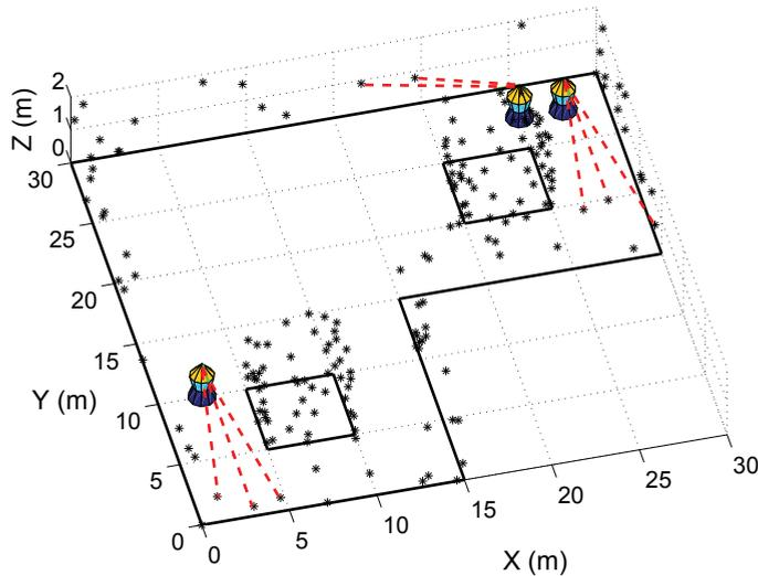
Fig. 5. Simulated environment. The robots perform observations of simulated landmarks located in walls. These walls are represented by a line. It can be observed that the walls restrict the visibility of the visual landmarks placed behind.
