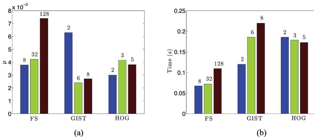
performance in accuracy for the three methods, even in the worst case. The  $\mu$  factor is lower than 0.0075 in all the cases. We must take into account that the  $\mu$  factor we get by using only the internal odometry without our algorithm is around 0.1421. With respect to the time  $t$ , FS clearly improves the other two descriptors. Anyway, with all three descriptors it is possible to work in real time since the times obtained are under 0.25 sec per iteration.
