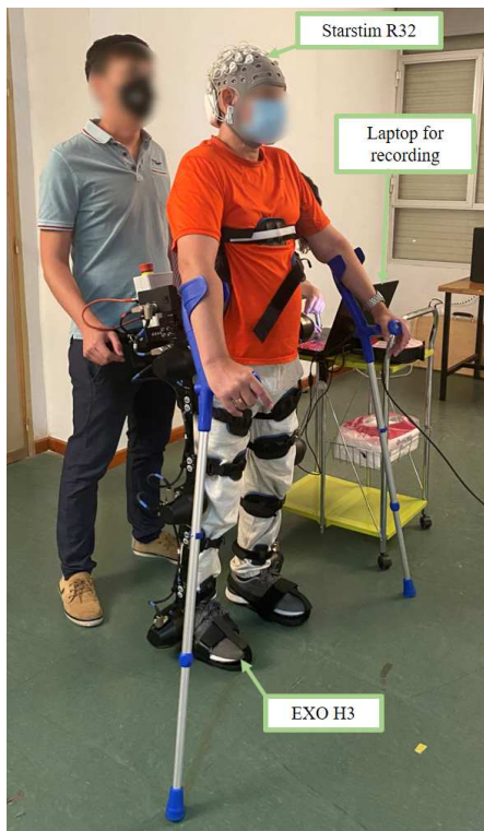
Figure 1. Experimental setup. The subject is depicted standing still while wearing the H3 exoskeleton with crutches and a Starstim R32 cap that records the EEG signal.
