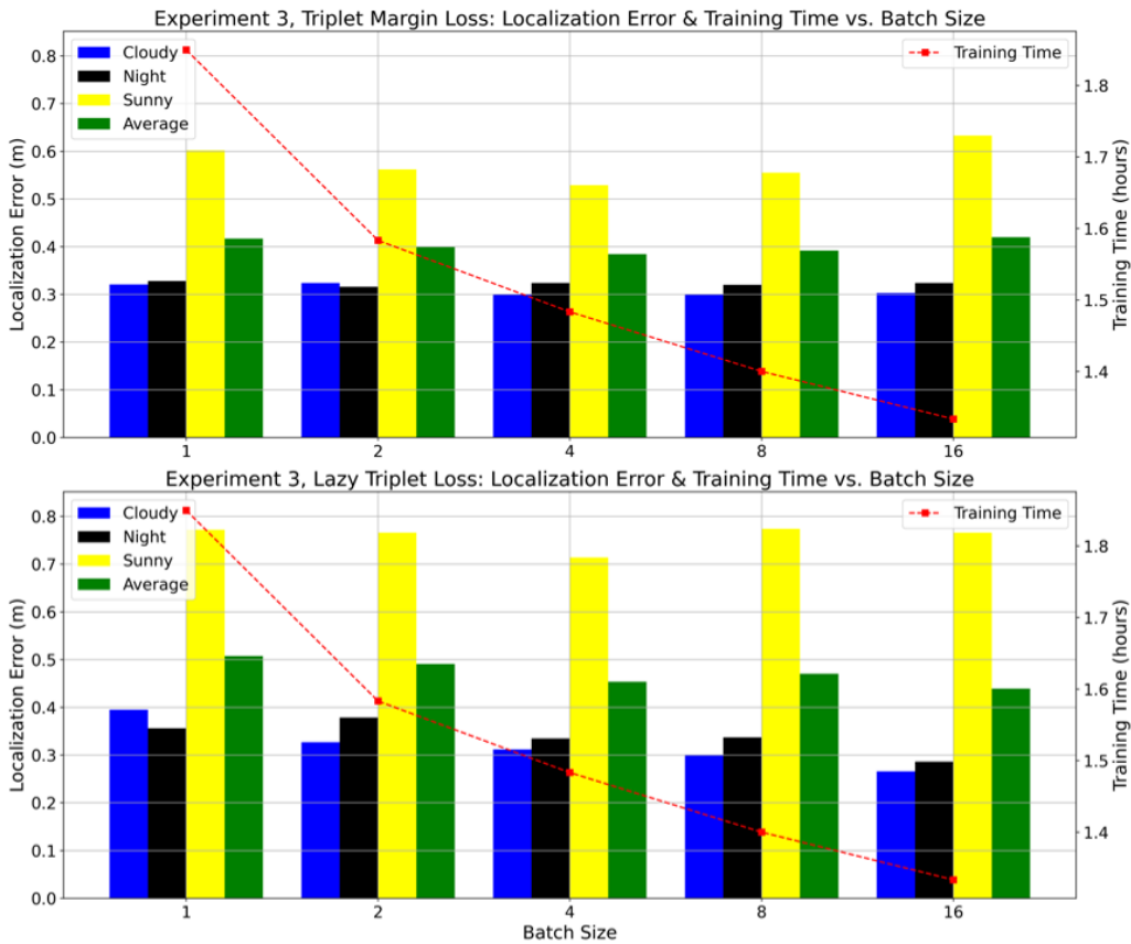
Figure 9: Comparison between the localization error and the training time versus the batch size in Experiment 3, with the Triplet Margin Loss (above) and the Lazy Triplet Loss (below).
