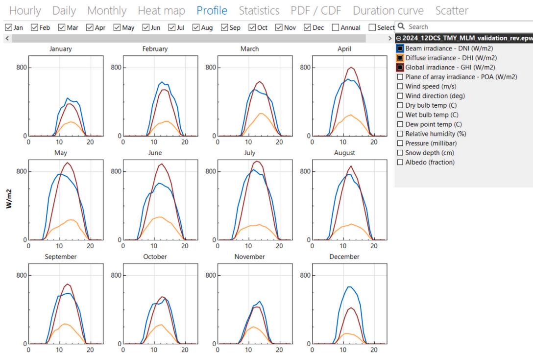
Fig. 4. Monthly hourly profiles of beam, diffuse, and global irradiance at the Enerstar-Villena CSP plant throughout 2024.
