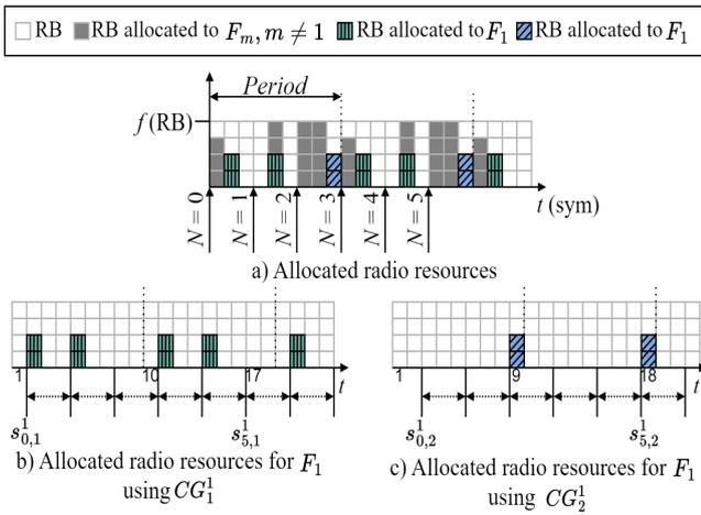
**Figure 2:** Example of the CG configuration definition and the use of the activation vector.
