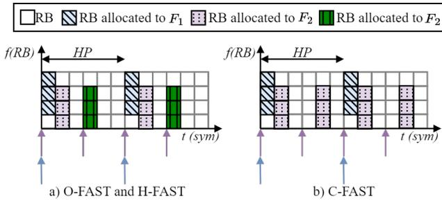
**Figure 3:** Example of scheduling solution when applying H-FAST, O-FAST and C-FAST.
