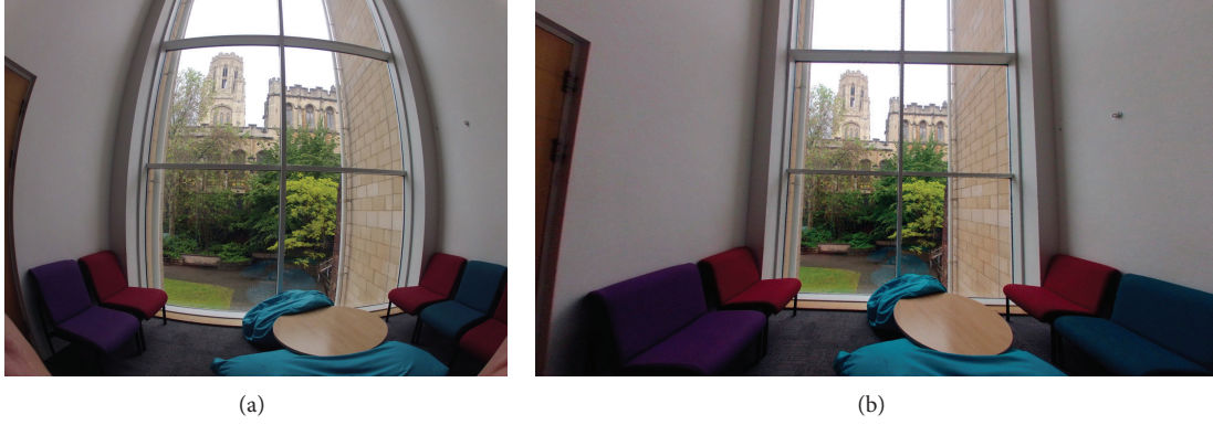
FIGURE 2: (a) Image captured with a fisheye lens camera and (b) its corresponding undistorted view.
