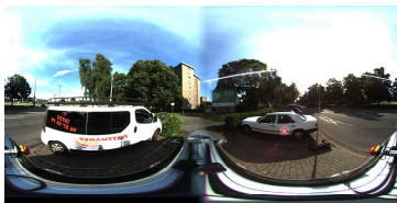
Figure 6: An equirectangular image generated from a pair of fisheye images of the KITTI-360 dataset (Liao et al., 2023).
