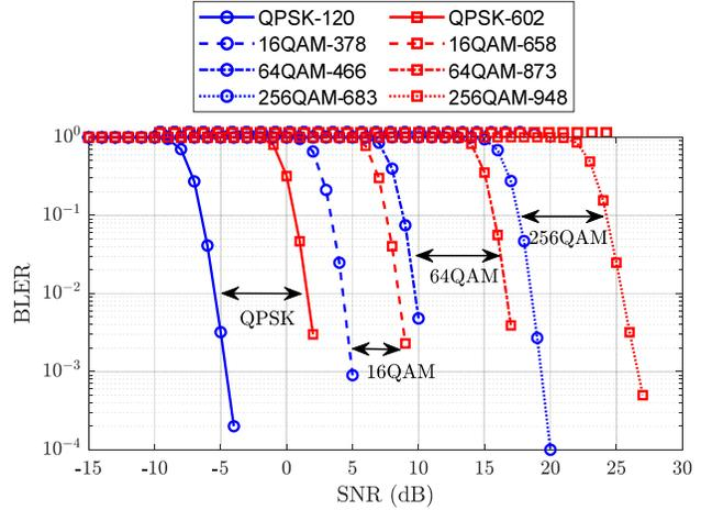
Fig. 8. Impact of the MCS on the TB BLER performance as a function of the SNR.
