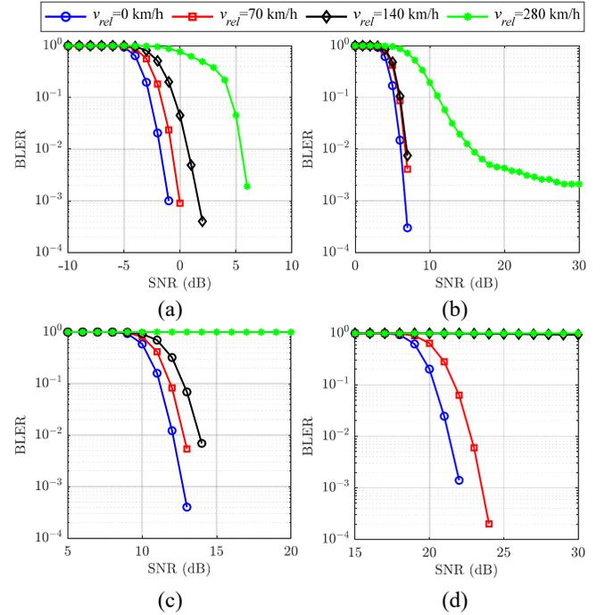
Fig. 5. Impact of the Tx–Rx relative speed on the TB BLER for different TB MCSs. (a) QPSK-308. (b) 16QAM-490. (c) 64QAM-616. (d) 256QAM-797.
