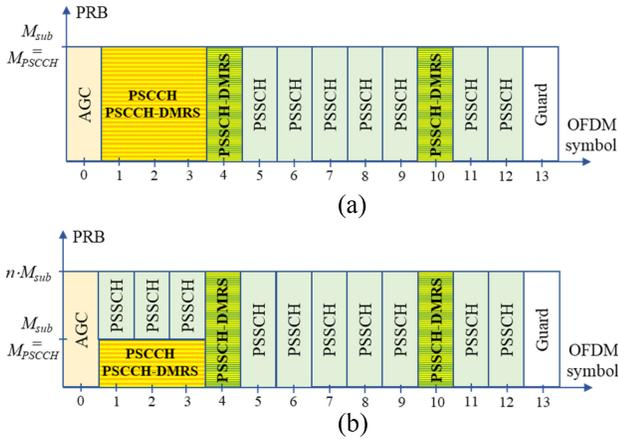
Fig. 1. PSSCH and PSSCH multiplexing in NR V2X SL: Normal CP, three PSCCH OFDM symbols, and two PSSCH-DMRS symbols. (a) 1 subchannel. (b)  $n$  subchannels.
