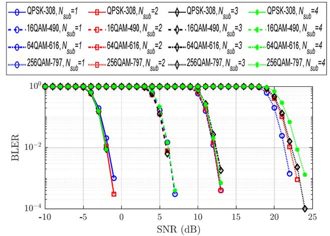
Fig. 9. Impact of  $N_{\text{sub}}$  on the TB BLER performance.
