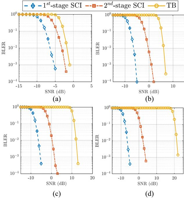
Fig. 4. First-stage SCI, second-stage SCI, and TB: BLER versus SNR curves for different TB MCSs. (a) QPSK-308. (b) 16QAM-490. (c) 64QAM-616. (d) 256QAM-797.
