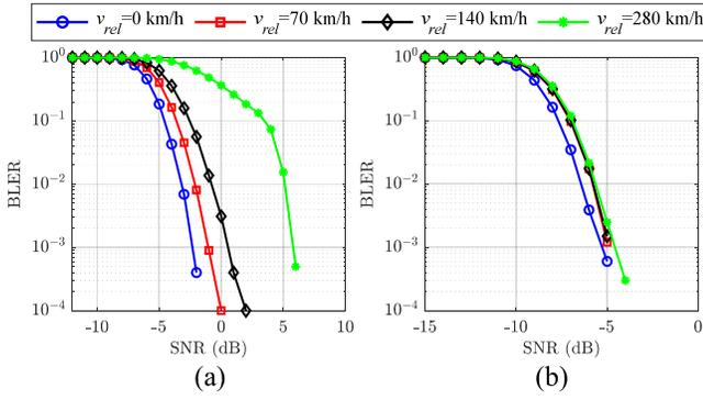
Fig. 6. Impact of the Tx-Rx relative speed on the second-stage SCI and first-stage SCI BLER. (a) Second-stage SCI. (b) First-stage SCI.
