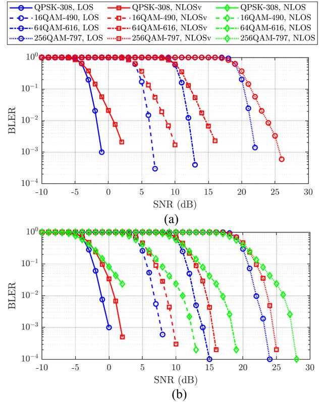
Fig. 7. TB BLER as a function of the SNR for different channel models and states. (a) Highway. (b) Urban.
