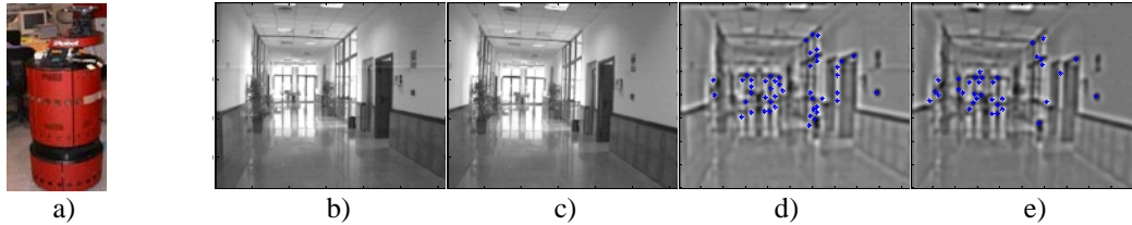
Fig. 1. Image (a) shows our B21r robot. Figures (b) and (c) show two images taken from our environment. Figures (d) and (e) show SIFT features extracted from them.
