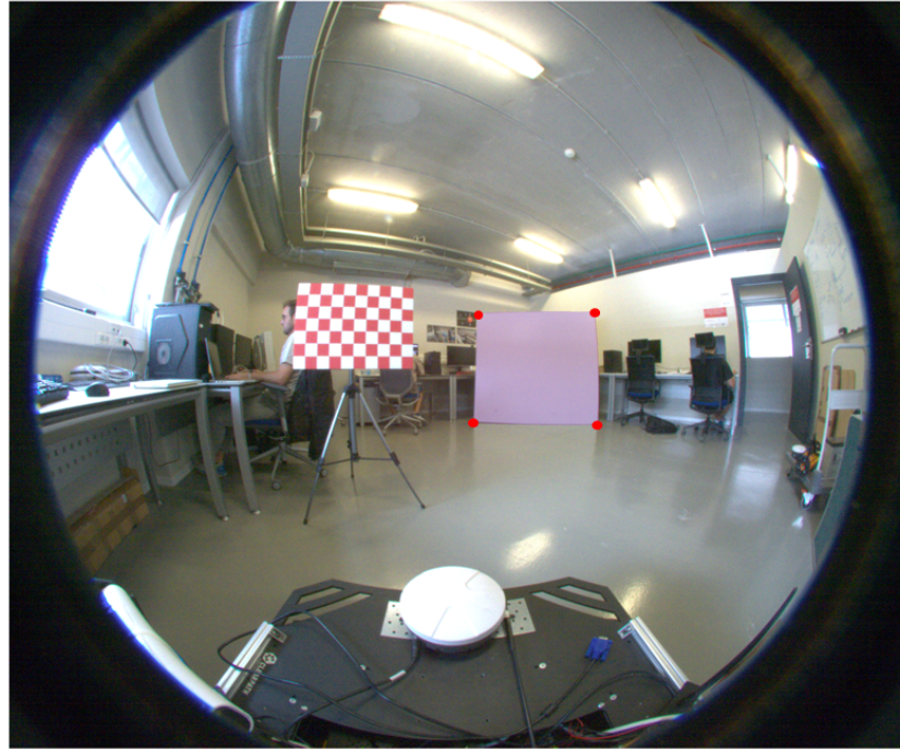
Figure 6. Image captured by the fisheye camera with the calibration rectangle segmented. The corners of the rectangular polygon are shown in red.
