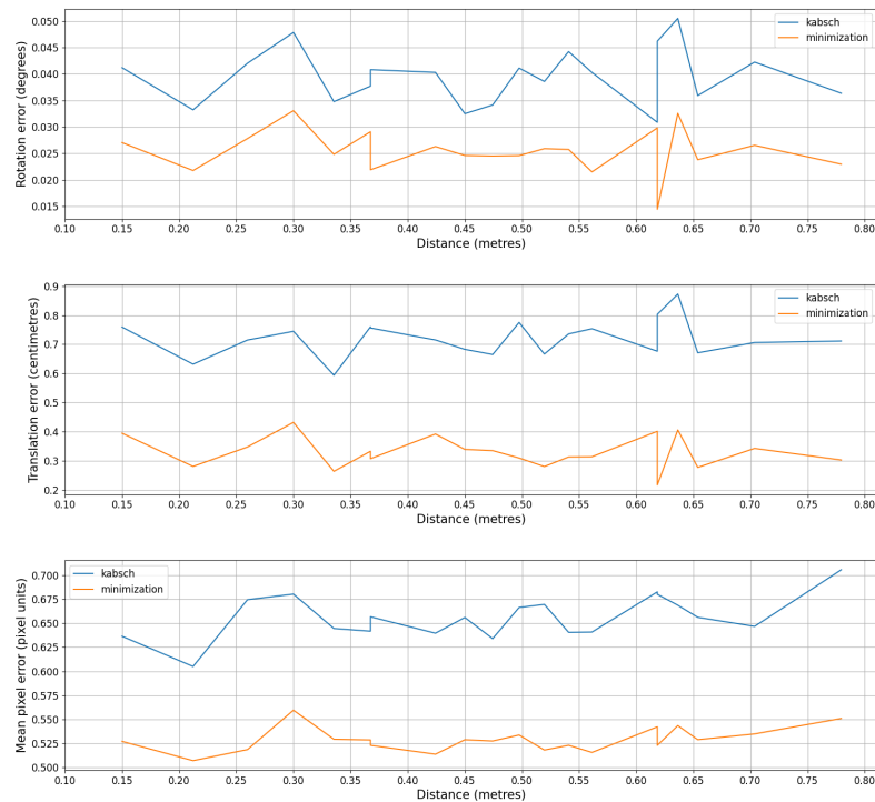
Figure 10. Rotation, translation, and mean pixel error versus distance between camera and LiDAR.
