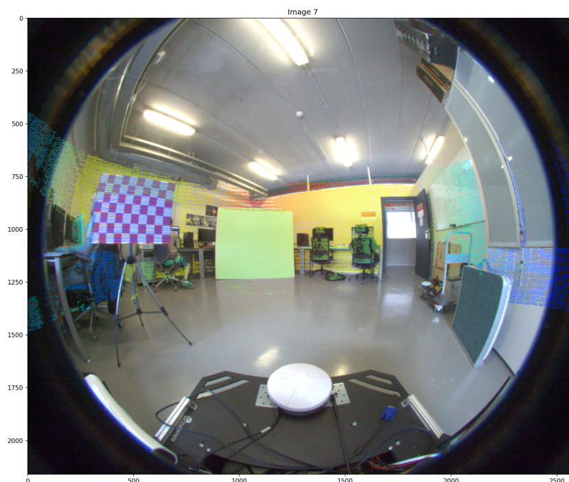
Figure 12. Point cloud projected onto the fisheye image after calculating the transformation between both systems with the minimization method. The color of the points is based on the distance from the camera, so the points closer to the camera are shown in blue and the points further away are shown in red.
