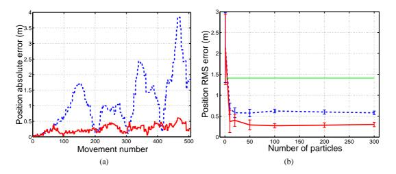
Figure 7: Figure 7(a) shows the absolute position error during the SLAM process. The final error in position is 0.34m. Figure 7(b) shows results in localization error when varying the number M of particles. The RMS error in odometry is shown as a dotted line. Results using equation (7) are shown as a dashed line and results using equation (8) are shown as a continuous line.
