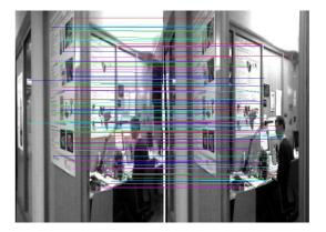
Figure 3: Stereo correspondences using SIFT features. The epipolar constrain is used to find correspondences across images.
