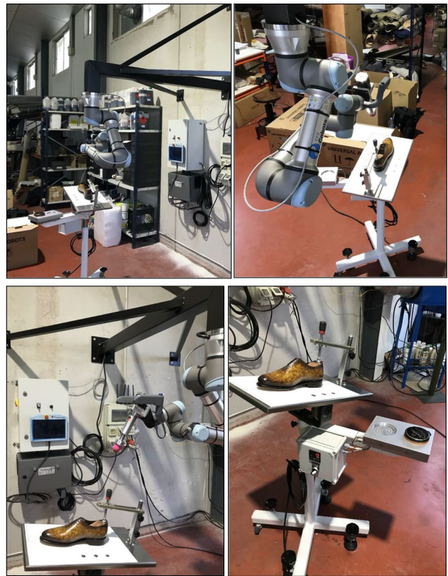
Fig. 12 Prototype of functional robotized cell for patina application
